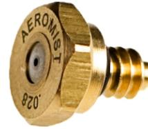
Orifices are machined from quality 316L Stainless Steel with the newest Swiss made CNC lathes to ensure precision, accuracy and consistency. Precise tolerances — not more than ± 7% flow variance per nozzle type. High quality O-rings offer leak-free performance.
