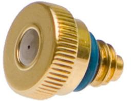
Orifices are machined from quality 316L Stainless Steel with the newest Swiss made CNC lathes to ensure precision, accuracy and consistency. Precise tolerances not more than  $\pm 7\%$  flow variance per nozzle type. High quality O-rings offer leak-free performance.
