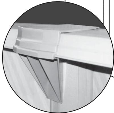
Hook the underside inside part of the top cover under the ledge as shown. Then lower the top cover until it rests evenly on the ledge. Place a 1/4"-14 x 1" self-tapping screw through the slot in the bottom cover and screw into the hole in the top cover. Be careful not to overtighten!
