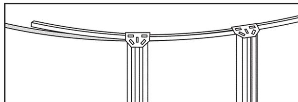
**MAKE SURE THAT THE TOP PLATE IS CENTERED DIRECTLY ON TOP OF THE BOTTOM PLATE.**
