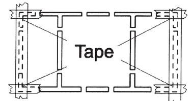
On inside of wall, tape over holes and slots that will not be used with duct tape or any other cloth tape.
