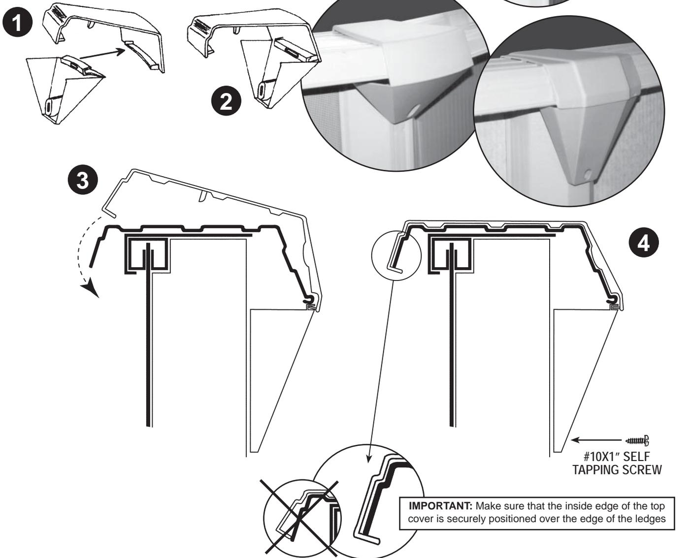
**IMPORTANT:** Make sure that the inside edge of the top cover is securely positioned over the edge of the ledges
