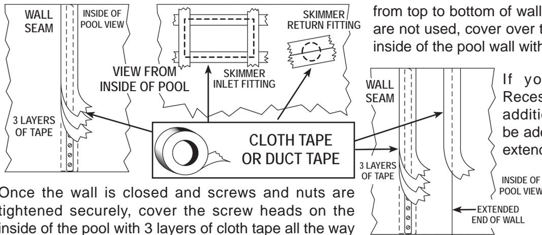
from top to bottom of wall. If the filter inlet and outlet are not used, cover over the pre-scored areas on the inside of the pool wall with 1 layer of tape.
