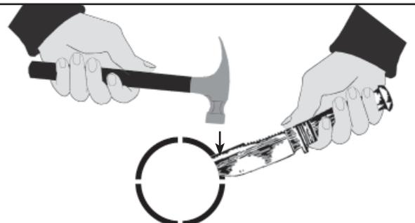
If the through wall filter inlet and outlet holes are to be used, remove metal cutouts by breaking perforations using a knife and hammer as shown. Refer to skimmer manufacturer's instructions for remainder of skimmer assembly. Make sure skimmer does not leak as this will corrode the pool wall and cause a split in the wall that is not covered under the pool warranty.
