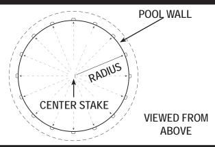
Using the center stake make sure your pool is completely in true round by measuring from the center of the stake to inside of pool wall in all directions, making sure these measurements are equal.
