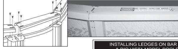
Place ledges over the wall with each end resting on a top plate. Using the above chart as a guide align the set of holes in the top plate as shown in the above drawing for your size pool with the holes in the ledge and insert the No.12x1/2" Sheet Metal Screw through the ledge and into the top plate. The actual screw holes that are used does not affect the integrity of the pool. You may use the set of holes that line up best!
