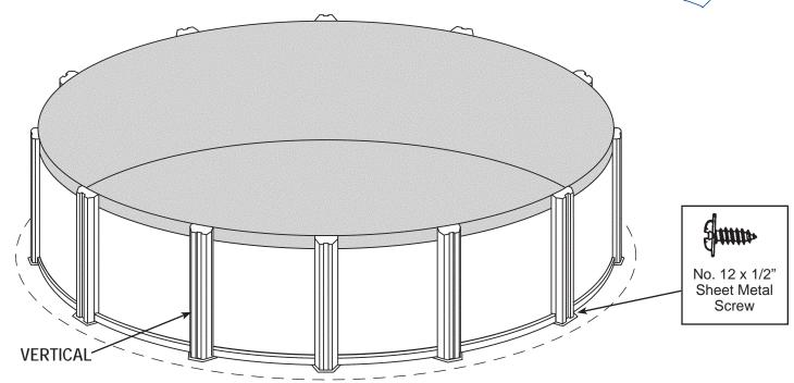
If fencing or decking is to be installed, refer to the deck and fence instructions before installing verticals. The holes indented in the face of the verticals must be on top.
