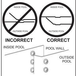
During the manufacturing process, the one end of the pool wall will have a slight crease or bend in it. Straighten out this bend as best as possible, and assemble the pool wall putting this end of the wall on the outside as shown.
