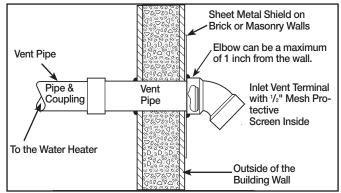
Figure 6 – Typical Horizontal Vent Installation
