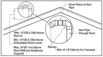
Figure 7 – Vertical Vent Terminal Location
