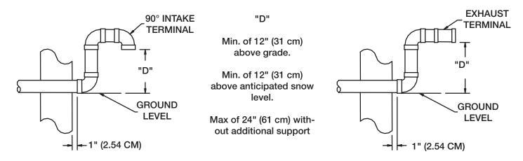
Figure 11a. Vent Terminal (Low Ground Clearance)
