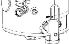
Figure 2 - Condensate Trap
