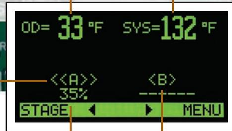
Boiler      Firing Rate      Lead Boiler (Indicated by parenthesis)
