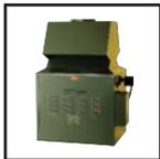
Rugged, outdoor proven even in the toughest environments, offers exceptional value while being the simplest unit to commission and maintain. With its atmospheric burner, horizontal water-tube design and standard Category I (B-vent) venting for indoor applications, installation is familiar and trouble-free.
