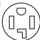
4-Wire Receptacle (14-30R)
