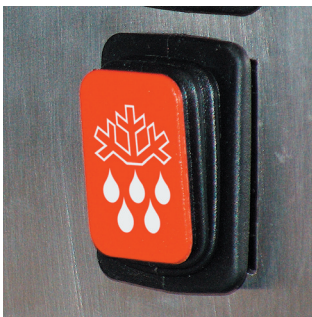
Hot Gas Defrost On-Demand Switch
