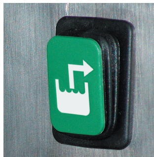
Pump Purge On-Demand Switch
