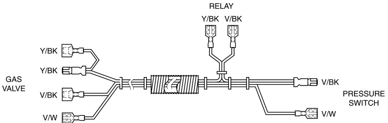
**Fig. 6: D-2 Power Vent Wire Harness**
